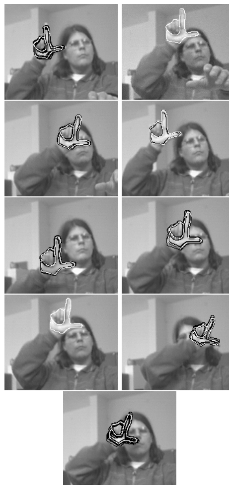
Fig. 3. Tracking hand in clutter with 100 particles. Black contours show particles having high observation likelihoods, whilst the white contour shows the actual estimate of the hand.
