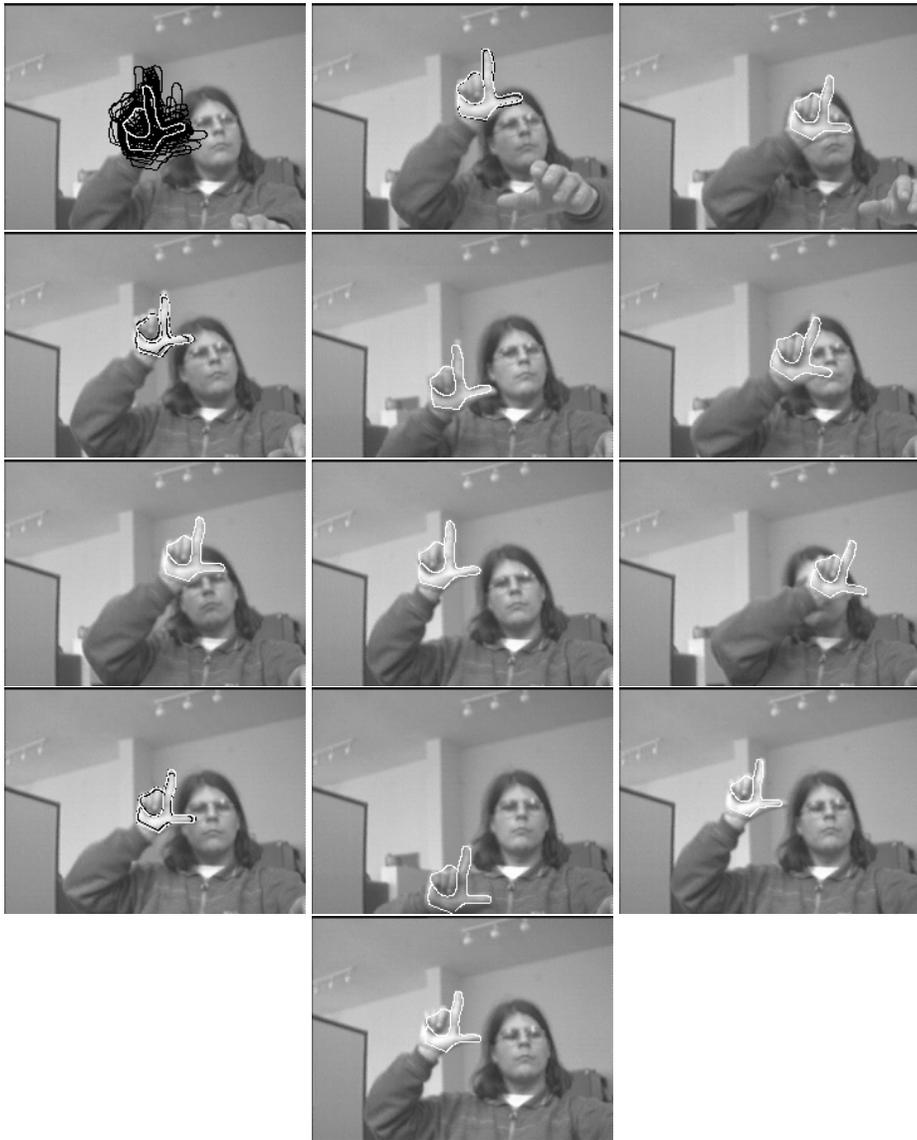
Figure 4: Tracking hand in clutter with 30 particles and the ANN0 method. Black contours show particles having high observation likelihoods, whilst the white contour shows the predicted contour of the hand. When no black contour is given, then typically there is only a single particle that has significantly higher likelihood than the others.
